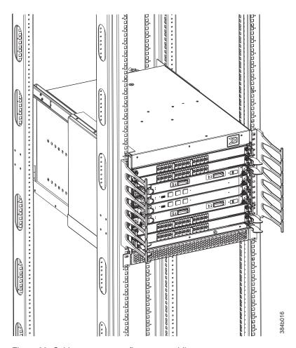
Figure 32. Cable management finger assemblies
